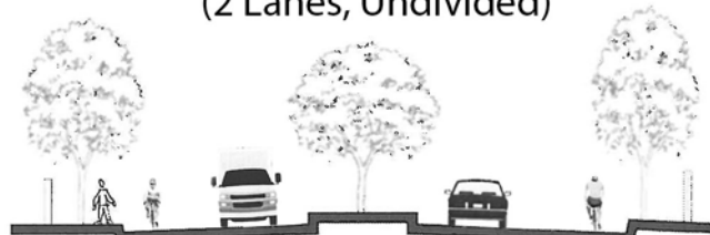
DIVIDED COLLECTOR ARTERIAL - 80' ( 2 Lanes, Undivided )
